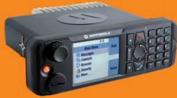
The **MTM5200** is the base model sharing the enhanced audio and receiver sensitivity of the current MTM5400, as well as being TEDS-ready.
