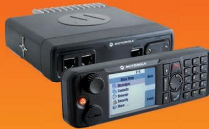
The **MTM5500** is a highly flexible and capable system radio which permits the installation of multiple control heads and/or the new Telephone Style Control Head up to 40m from the radio.
