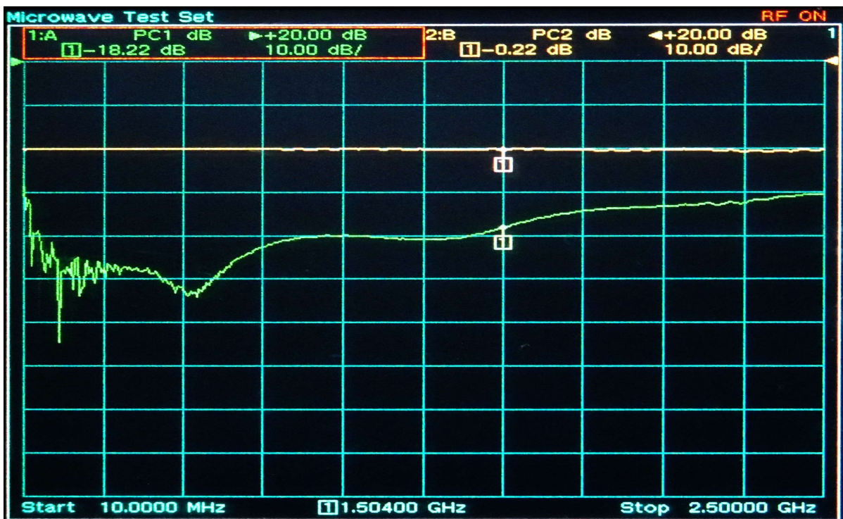
Fig. 3 Graph of attenuation/adaptation factors of surge protection SPKO-N-050-1,5G-B/F-M in the 10 MHz-2,5 GHz frequency band.
